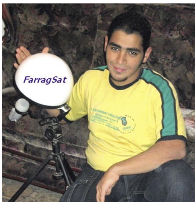
From Dr. Farrag's workshop: a 25cm half spherical mini antenna with external LNB presented by his son Kariem in their living room. Reception is possible starting with 50 dBW
