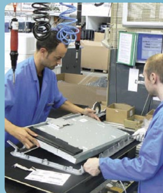
▲ The flat-screen LCD panels arrive and are placed on the main housing and are secured from behind: this is the first step in making it a complete unit.
