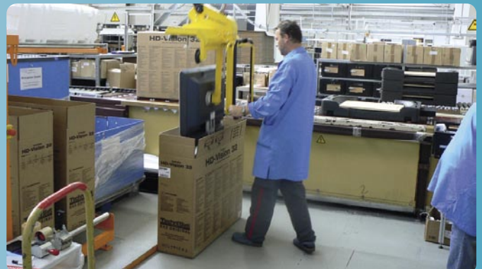
▲ The final step: a crane is used to lower the finished product into its shipping box – and that's it!
