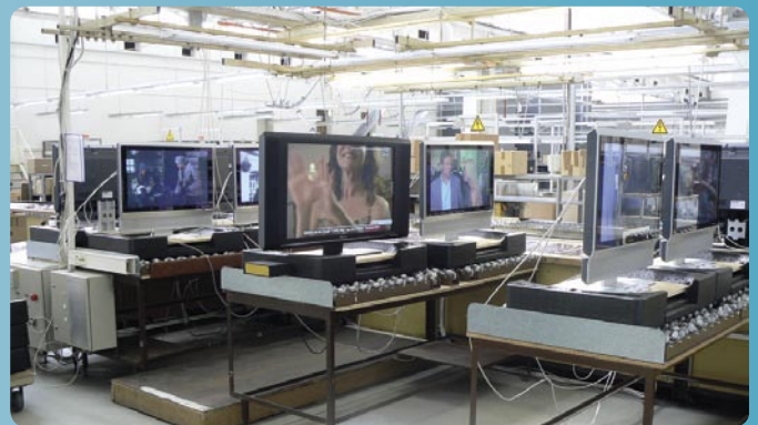
▲ After installing the speakers, the flat-screen LCD TV is ready to ship. A few sample units are taken out of the production line and placed on these test stands and put through a series of long-term tests.
