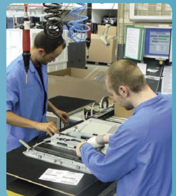
▲ The main board is placed on top of the LCD panel and secured in place with screws.
