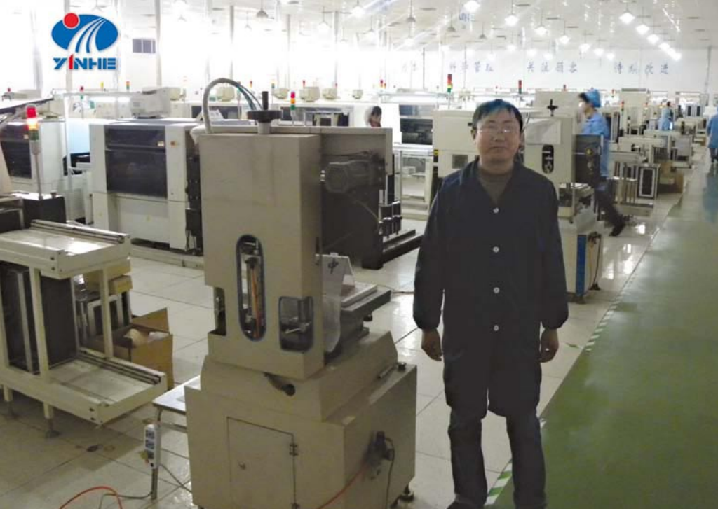
■ 11 production lines are in the SMT room. Qian Ming is in charge here and tells us, "We operate with two Yamaha SMT automated machines, six from Juki, two from Panasonic as well as a line for tests and repairs. With these automated machines we can produce seven million pieces a month."
