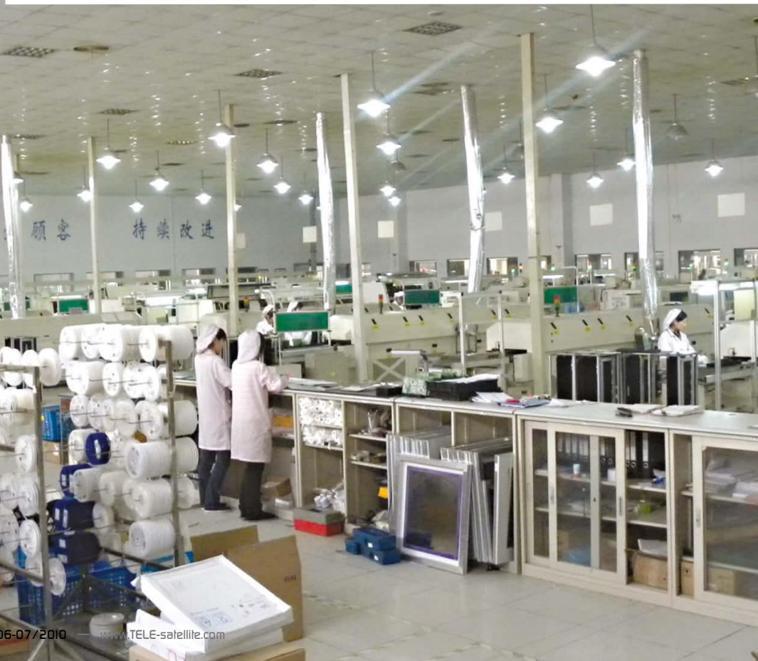
■ At the other end are the rolls with the surface mount components. They are continuously fed by an employee into the SMT automatic mounting machines. The SMT automatic machines run 24 hours a day. The Chinese writing on the wall in the background reads: "Work with Your Fellow Employees; Good Management; Customer Orientation; Continuous Improvement".
