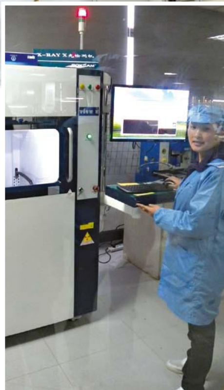
■ Faults are examined in a separate clean room. This is where a BOXSAM employee uses X-rays to detect any deficiencies.
