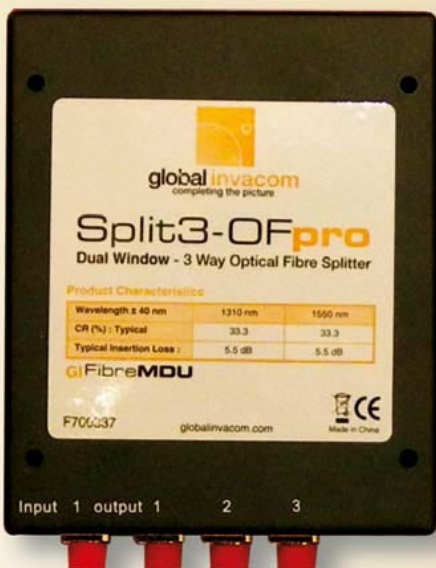
■ GlobalInvacom modified the optical splitter with connector jacks: the optical connection cables can now be directly plugged into the splitter.
