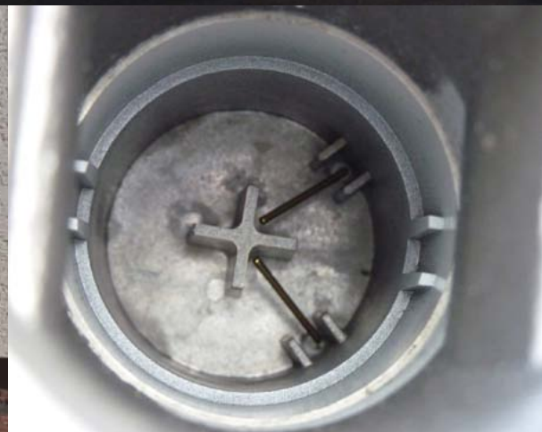
■ A look inside the AVCOM LNB: Only the cross-shaped element in the background is rotated. Depending on the 45° turn either linear or circular signals can be received.
