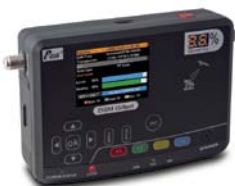
8DTEK DSM GIFTED Satellite Meter for Antenna Alignment ..... 30
