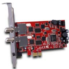
SATCATCHER DIGIPRO ST COMBO Combination Signal Analyzer for DVB-S and DVB-T ..... 62
