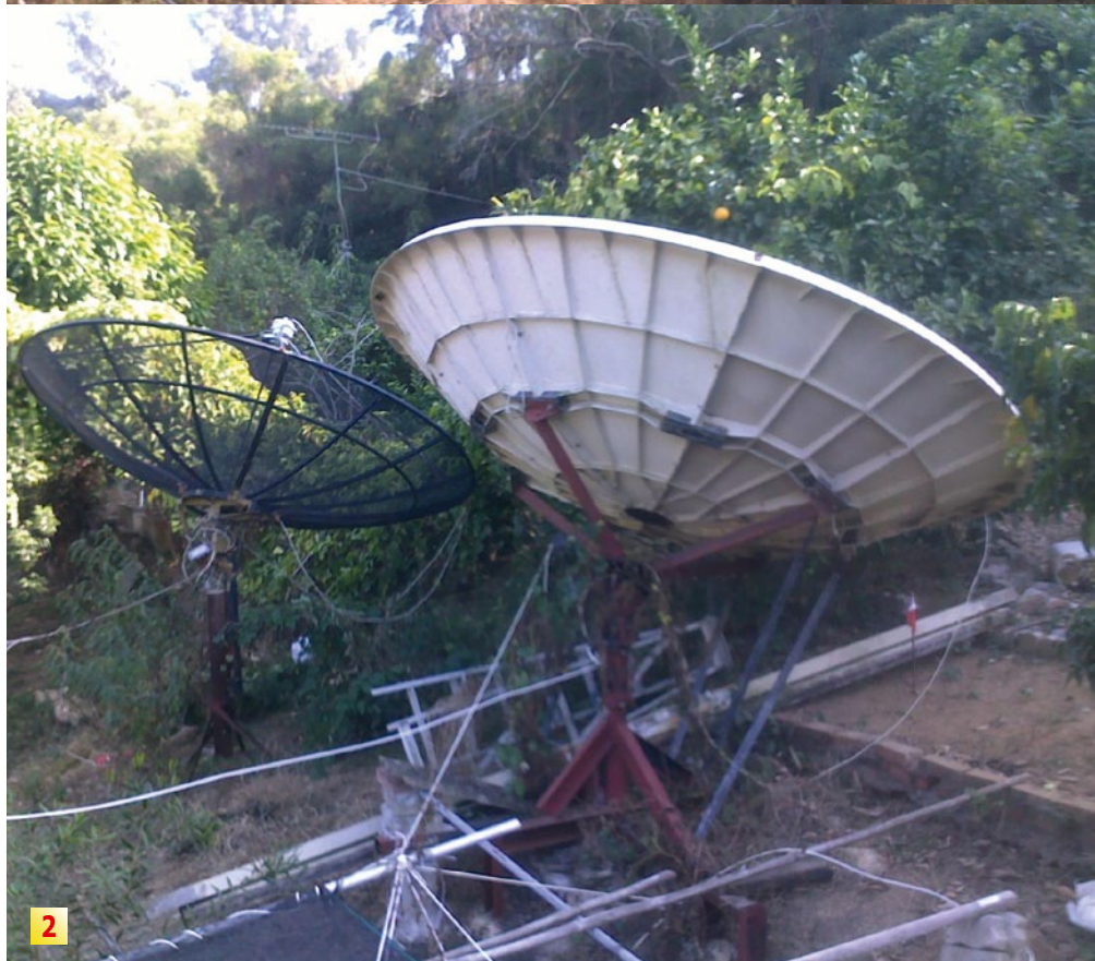
1. This is one of Ken Wong's 3-meter antennas with a motor on one of Kong Kong's islands.
