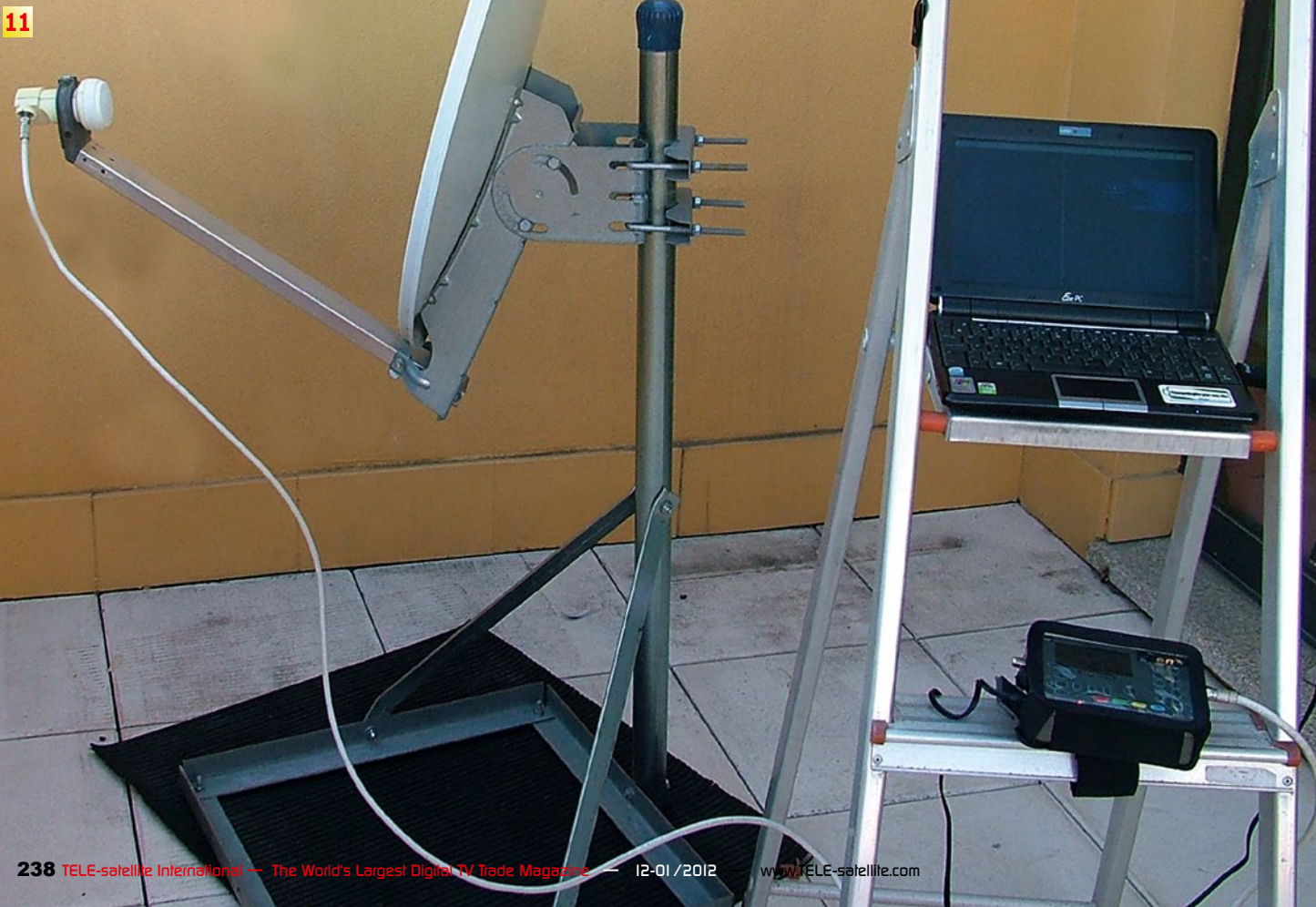
Image 11: Second test set-up, this time using a netbook and the Desired. Long-term measurement tests were carried out with this equipment.
