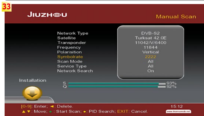
31. Channel list restriction to favorite lists 32. Channel list restriction to individual satellites 33, 34. SCPC reception via TURKSAT 42° East
