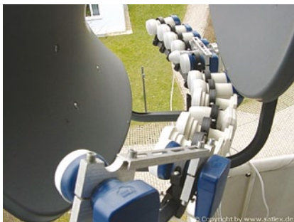
Assembly of additional LNB's
