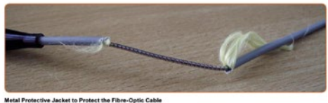
Metal Protective Jacket to Protect the Fibre-Optic Cable
