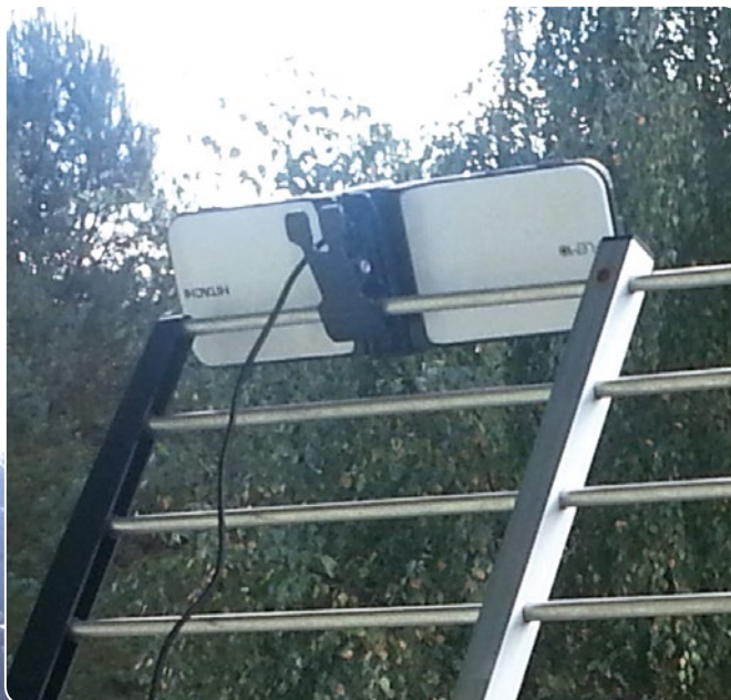
■ The FLEMO mounted on top of a full grown UHF antenna during our tests. Reception of the FLEMO is only 8 dB less compared to the big antenna.
