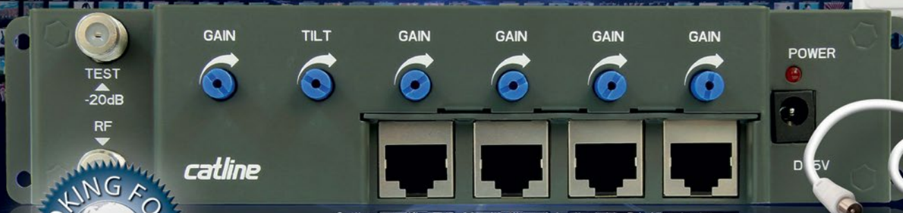
Catline amplifier TVB-02 with tilt and 4 adjustable RJ-45 outputs.
